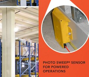
An infrared light beam, unaffected by sunlight or ambient light extremes, projected the length of the carriage at its base stops system movement when broken by a person's foot or other object.
