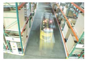
An **ActivRAC** System can be configured to your application with just one access aisle to accommodate existing fork trucks and pallet racks, to enhance your productivity and reduce driver damage. A fast aisle-opening cycle time helps you maintain or improve your throughput of puts and picks.
